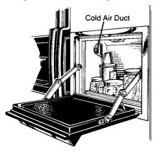
Cold air entering from the freezer compartment keeps the temperature in the Countermaker Compartment at proper food-keeping levels.
